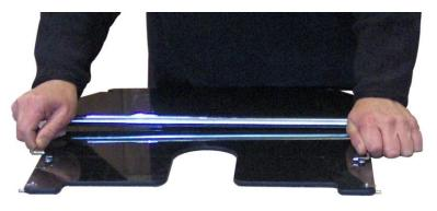
**25.** Remove the Shelf Supports from all six Feed Shelves by spreading the rod from the loop straps.
