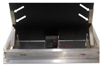
**14.** Install four 10-32 x  $\frac{1}{2}$ " screws through the holes in the Door Sides and the Back Stop. Install a 10-32 lock nut on each screw and tighten.
