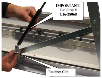
9. Remove the retaining clips from the ends of the Struts. Install the Strut with part # C16-28068 first. Be sure to install it exactly as shown (shaft end up). First attach the barrel end to the frame. Next attach the shaft end to the linkage. Be sure retaining clips snap firmly into place.
