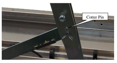
**8.** Insert the cotter pin through the hole in the 5/16 pin. Spread the cotter pin to secure it in place.
