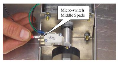
**17.** Attach the black wire from the Control Panel to the middle spade on the white micro-switch. The bottom spade on the micro-switch will be left blank.
