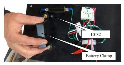
**21.** Attach the Battery Clamp to the back of the Control Panel by inserting two 10- $32 \times \frac{3}{4}$ " screws through the holes just to the right of the Timer. Thread the screws partially into the Battery Clamp but do not tighten. Do not install the battery (included) at this time.
