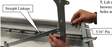
**7.** Lift the Straight Linkage into place between the Door Linkages. Align the holes and insert the 5/16" pin.
