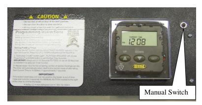
31. Test the connections by pressing the manual switch, the camshaft should begin to rotate. Continue to press the manual switch for two seconds then release. The camshaft should continue until it completes a 180° rotation. The camshaft should rotate in a counter clockwise direction when looking at it from the Control Panel end. If it rotates the wrong direction, check the positive and negative connections on the battery.
