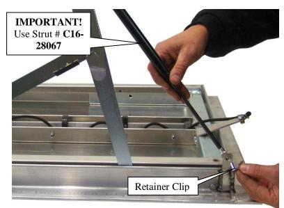
10. Now install the Strut with part # C16-28067. Be sure to install it exactly as shown (shaft end down). First attach the shaft end to the frame. Next attach the barrel end to the linkage. It may be necessary to compress the Strut slightly. Be sure retaining clips snap firmly into place. \*\*\*IMPORTANT: The Struts have different pressure amounts and must be installed in the correct positions. If installed incorrectly the door will not open and close properly.\*\*\*
