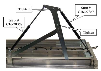
**11.** Your strut and linkage assembly should now look exactly like this. Tighten the two 5/16 hex bolts and nuts that were installed in steps 5 & 6.
