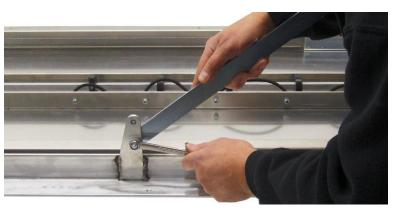
**4.** Slide the Straight Linkage stud through the 5/16" hole in the frame. Install another nylon washer and a ½" lock nut and tighten. Be sure the nylon washer fits over the shoulder on the Straight Linkage stud. The straight linkage should pivot freely when finished.
