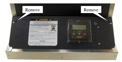
**29.** Remove the two 10-32 screws holding the Control Panel. Tip the Control Panel towards you to reveal the back side.
