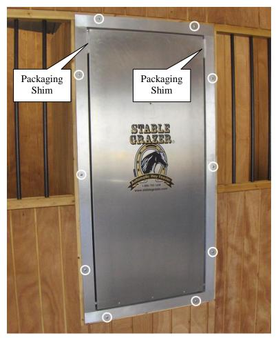
23. Leave the packaging shims in place for this step. While being careful not to let the door open in the frame set the feeder into your enclosure. Using appropriate fasteners (not included) attach it to your structure through the holes in the door frame as indicated by the white circles.
