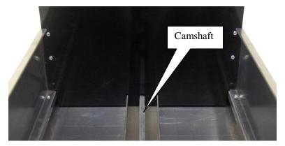
**15.** The Back Stop will shift slightly from side to side. Center the hole in the Back Stop over the camshaft and tighten all the screws and bolts installed in step 12.
