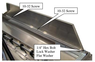
**12.** Attach the left Door Side to the door using two 10-32 x ½" screws and a 1/4" x 1" hex bolt with lock washer and flat washer. Do not tighten at this time. Repeat for the right Door Side.
