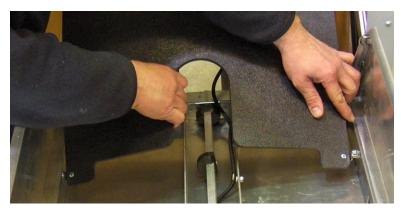
26. One Feed Shelf is shorter than the other five, start with this shelf. While standing on the left side of the door and starting from the end furthest from the Control Panel, install the Feed Shelves with the textured side up. Place the hinge pin in the first hole nearest you then flex the shelf enough to insert the opposite hinge pin in the corresponding hole on the opposite side. Continue until all the Feed Shelves are installed.
