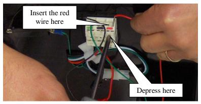
19. Using the same method as above attach the red wire from the motor to the terminal block on the Control Panel.
