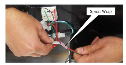
**20.** Group the red, green and black wires together. Re-install the spiral wrap around these three wires.
