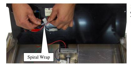
**16.** Remove the spiral wrap from the wires on the back of the Control Panel. **Note:** The Back Stop has been removed in steps 16 – 21 for clarity.
