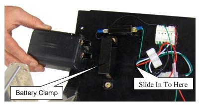
**30.** Slip a 6 Volt screw terminal battery (included) into the Battery Clamp. Slide it in until it just touches the wires coming through the Control Panel. Tighten the two 10-32 screws holding the Battery Clamp until the battery feels snug. Attach the wires to the battery terminals. Take special care to attach the red wire to the positive (+) and the black wire to the negative (-) terminals. **Note:** The Back Stop is removed for clarity.
