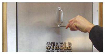
**24.** Attach the handle to the feeder door using two 10-32 x  $\frac{1}{2}$ " screws.
