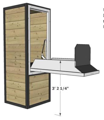
Using the recommended Dimension C will leave you with approximately 3' 2 <sup>1</sup>/<sub>4</sub>" from the floor to the top of the door side when the feed door is in the load position.
