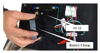
**21.** Attach the Battery Clamp to the back of the Control Panel by inserting two 10- $32 \times \frac{3}{4}$ " screws through the holes just to the right of the Timer. Thread the screws partially into the Battery Clamp but do not tighten. Do not install the battery (not included) at this time.
