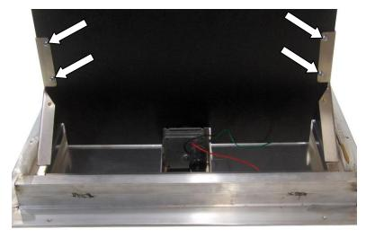
**14.** Install four 10-32 x  $\frac{1}{2}$ " screws through the holes in the Door Sides and the Back Stop. Install a 10-32 lock nut on each screw and tighten.
