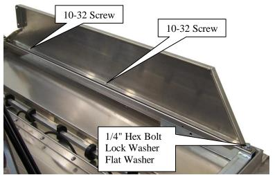
**12.** Attach the left Door Side to the door using two  $10-32 \text{ x } \frac{1}{2}$ " screws and a  $\frac{1}{4}$ " x 1" hex bolt with lock washer and flat washer. Do not tighten at this time. Repeat for the right Door Side.
