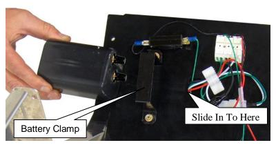
30. Slip a 6 Volt screw terminal battery (not included) into the Battery Clamp. Slide it in until it just touches the wires coming through the Control Panel.
